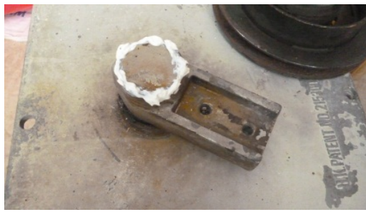
Silicone is used to glue the belt tensioner to the motor
