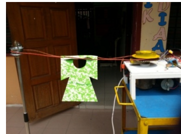
The microphone stand is placed away from the trolley and a leather treadle belt is looped through the car belt tensioner and tire rim making a clothesline.
