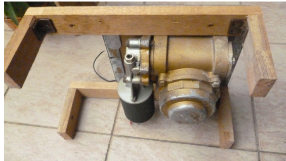
Bed frame is chopped and stuck to four corners of the motor's base.
